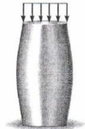
Compression causes material to bulge out
